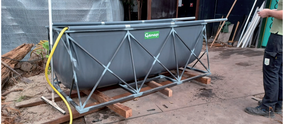
Fig. 3: The TAP is mounted in a metal frame. It is pre-filled to 45 cm of water. Measurements of the TAP are a length of 245 cm on the top, 200 cm at the bottom. Width and height of the Tap are 80 cm. The metal frame is 245 cm long and 90 cm high, with a width of 80 cm on the top and 120 cm at the bottom. Photo: R. Bernhard.
