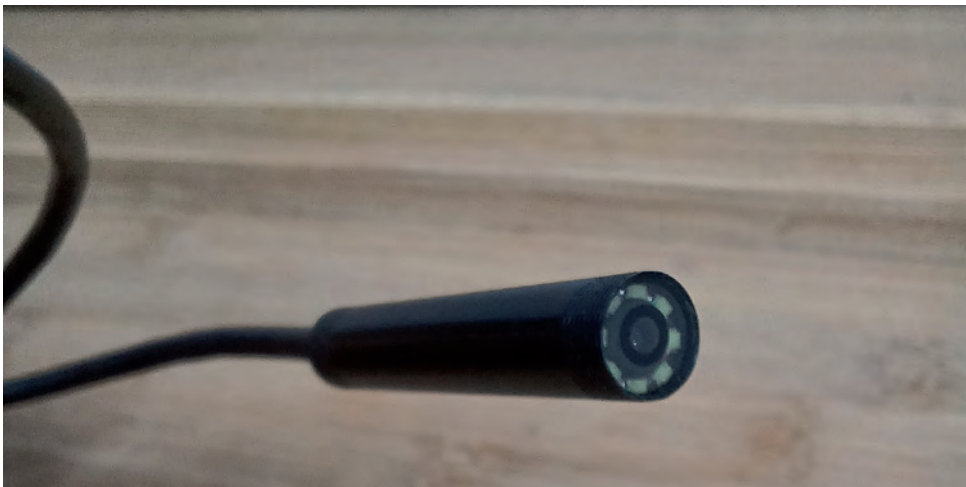
Fig. 4: Endoscope camera used for looking into the nest without destroying it. Photo: T. Breuer
